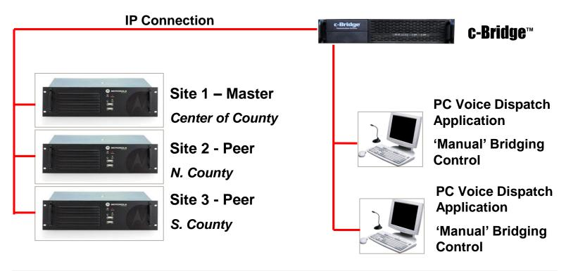
The **C-Bridge**™ can be used as an "IP Gateway", allowing for IP-based Remote Voice Dispatch, where control stations or tone-control systems are not needed
