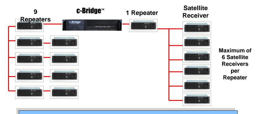
A **c-Bridge**<sup>™</sup> can be used to expand this limit to 6 Satellite Receivers per Repeater
